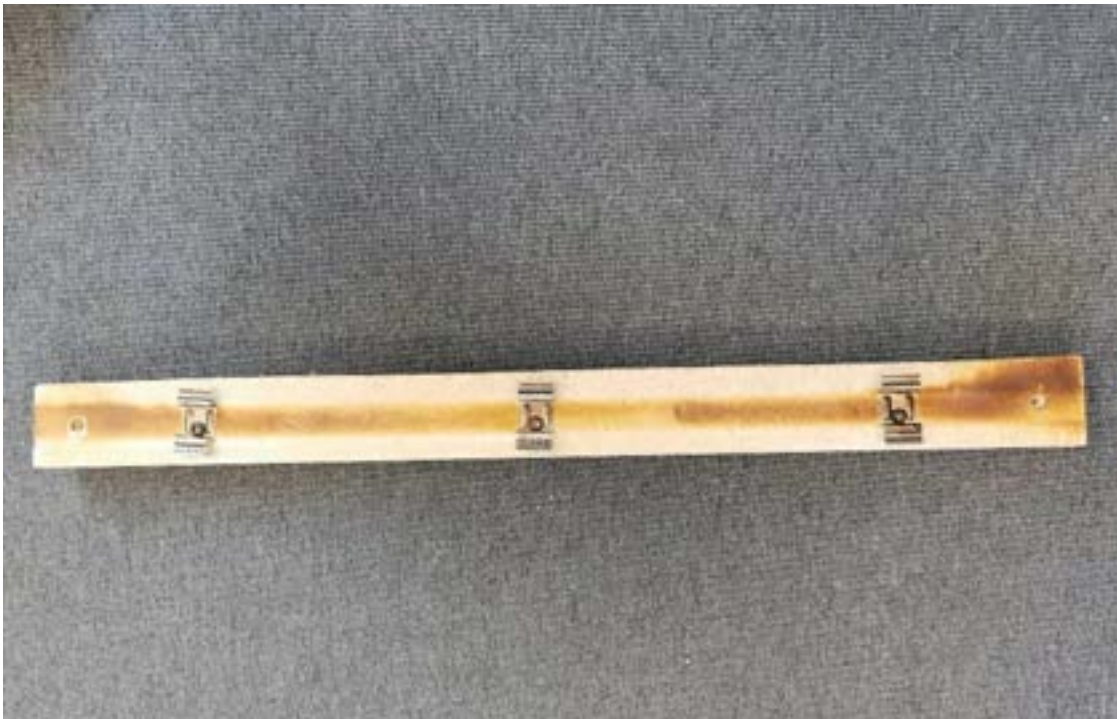
Photo No. 2 Damages on the wooden lath
